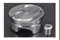
Compared with the removal of the secure yet unwieldy spiral locks or round wire locks, changing buttons is remarkably convenient. In addition, on pistons where the pin bores intercept the oil control ring groove, the buttons prevent the expander in the oil control ring from distorting around the half moon openings in the back of the groove, a deficiency more prevalent in power adder engines.
