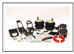
Designed to mount between the truck's frame and the suspension, Firestone's Ride-Rite kits use air pressure to help maximize the truck's safe load carrying capacity, stability and ride quality. Featuring individual inflation valves for separate side-to-side or front-to-rear adjustment, the air helper springs also assist in leveling off-center loads.
