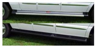
Owens' new Thermoplastic Polyolefin (TPO) molded board is available in both 100" and 120" and comes with a full-length, galvanized steel support which provides durability and serviceability. These TranSender boards have a tread design embedded in the TPO, providing secure footing year around with flair.
