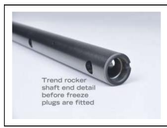
Created to overcome deflection and to improve valve-train stability when used in conjunction with high-performance camshafts and valve train, Trend produces this new shaft from thickwall 4130 chrome molybdenum, subjects it to two heat treatments-through-hardening and nitriding-and finally applies a DLC (diamond-like coating).
