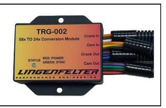
model GM engine applications. The product features a fully encapsulated (potted) construction for increased durability and a high temperature glass-filled Nylon low-profile case. Transient voltage and over-voltage protection have been incorporated into the design to accommodate the ever-increasing electrical demands of modern vehicle control systems. It also incorporates a bi-color LED to indicate the operating status.
