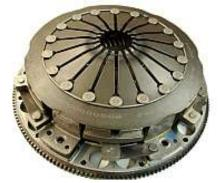
The Lingenfelter 6-bolt flange flywheel is an OEM spec steel design created specifically to accept the production 2009 General Motors ZR1 Corvette dual disk clutch pressure plate assembly. This allows the ZR1 clutch to be installed on LS2, LS3
